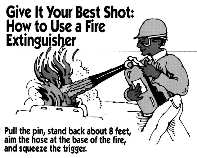
Make sure your first shot is on target—the fire extinguisher only lasts 3 to 20 seconds.
